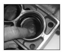
Place support ring (41) and v-sleeves (40) into valve casing (43).
